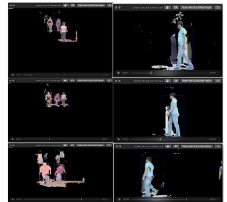
FIGURE 5.6: Tracking with background subtraction
